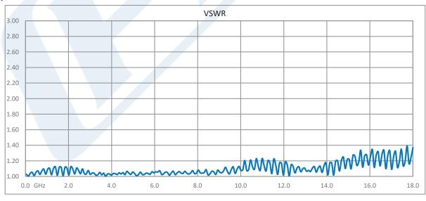
Click the following link (or enter part number in "SEARCH" on website) to obtain additional part information including price, inventory and certifications: SMA Female Bulkhead to SMA Female Bulkhead Low Loss Cable 150 CM Length Using PE-P160LL Coax PE3C5247-150CM
