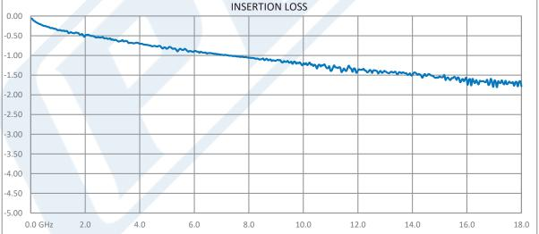
Click the following link (or enter part number in "SEARCH" on website) to obtain additional part information including price, inventory and certifications: SMA Male Right Angle to SMA Female Bulkhead Low Loss Cable 36 Inch Length Using PE-P160LL Coax PE3C5244-36
