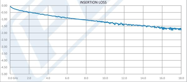
Click the following link (or enter part number in "SEARCH" on website) to obtain additional part information including price, inventory and certifications: SMA Male Right Angle to SMA Female Bulkhead Low Loss Cable 200 CM Length Using PE-P160LL Coax PE3C5244-200CM
