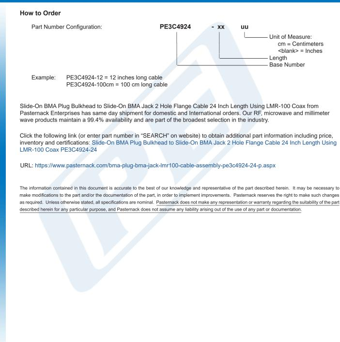
Pasternack Enterprises, Inc. • P.O. Box 16759, Irvine, CA 92623 **Phone:** (866) 727-8376 or (949) 261-1920 • **Fax:** (949) 261-7451 Sales@Pasternack.com • Techsupport@Pasternack.com PE3C4924-24 CAD Drawing Slide-On BMA Plug Bulkhead to Slide-On BMA Jack 2 Hole
