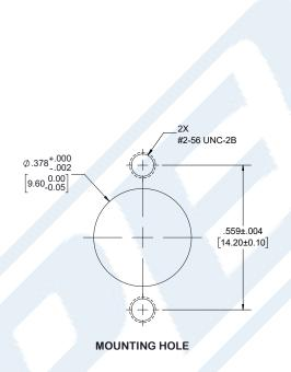
Click the following link (or enter part number in "SEARCH" on website) to obtain additional part information including price, inventory and certifications: Slide-On BMA Jack 2 Hole Flange to SMA Male Right Angle Cable 24 Inch Length Using RG405 Coax PE3C4885-24
