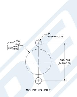
Click the following link (or enter part number in "SEARCH" on website) to obtain additional part information including price, inventory and certifications: Slide-On BMA Jack Right Angle 2 Hole Flange to Slide-On BMA Jack Right Angle 2 Hole Flange Cable 36 Inch Length Using RG405 Coax PE3C4876-36
