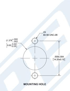
Click the following link (or enter part number in "SEARCH" on website) to obtain additional part information including price, inventory and certifications: Slide-On BMA Jack 2 Hole Flange to Slide-On BMA Jack 2 Hole Flange Cable 6 Inch Length Using RG405 Coax PE3C4873-6
