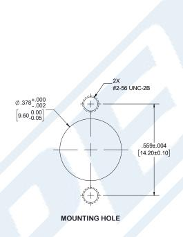
Click the following link (or enter part number in "SEARCH" on website) to obtain additional part information including price, inventory and certifications: Slide-On BMA Jack 2 Hole Flange to SMA Male Cable 12 Inch Length Using PE-SR405FLJ Coax PE3C4855-12
