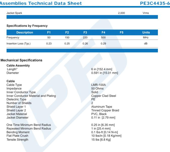
Click the following link (or enter part number in "SEARCH" on website) to obtain additional part information including price, inventory and certifications: SSMC Plug Right Angle to TNC Male Low Loss Cable 6 Inch Length Using LMR-100 Coax PE3C4435-6
