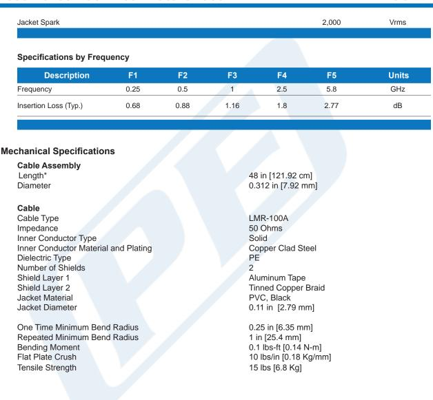
Click the following link (or enter part number in "SEARCH" on website) to obtain additional part information including price, inventory and certifications: SMA Female to SSMC Plug Low Loss Cable 48 Inch Length Using LMR-100 Coax PE3C4426-48
