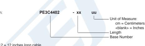
Example: PE3C4402-12 = 12 inches long cable PE3C4402-100cm = 100 cm long cable
