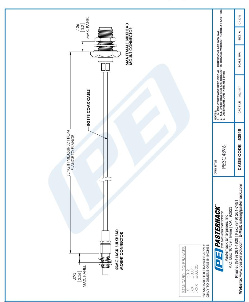
PE3C4396-72 CAD Drawing SMA Female Bulkhead to SSMC Jack Bulkhead Cable 72 Inch Length Using RG178 Coax
