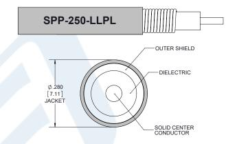
Click the following link (or enter part number in "SEARCH" on website) to obtain additional part information including price, inventory and certifications: Plenum 7/16 DIN Male Right Angle to 7/16 DIN Male Right Angle Low PIM Cable 36 Inch Length Using SPP-250-LLPL Coax , LF Solder PE3C4144-36
