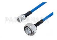
Plenum N Female to 7/16 DIN Male Low PIM Cable 50 CM Length Using SPP-250-LLPL Coax , LF Solder
