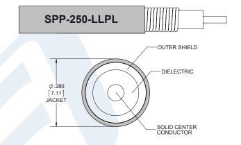
Click the following link (or enter part number in "SEARCH" on website) to obtain additional part information including price, inventory and certifications: Plenum 7/16 DIN Male Right Angle to 7/16 DIN Male Low PIM Cable 60 Inch Length Using SPP-250-LLPL Coax , LF Solder PE3C4131-60
