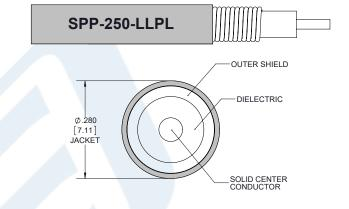
Click the following link (or enter part number in "SEARCH" on website) to obtain additional part information including price, inventory and certifications: Plenum 7/16 DIN Male Right Angle to 7/16 DIN Male Low PIM Cable 100 CM Length Using SPP-250-LLPL Coax , LF Solder PE3C4131-100CM
