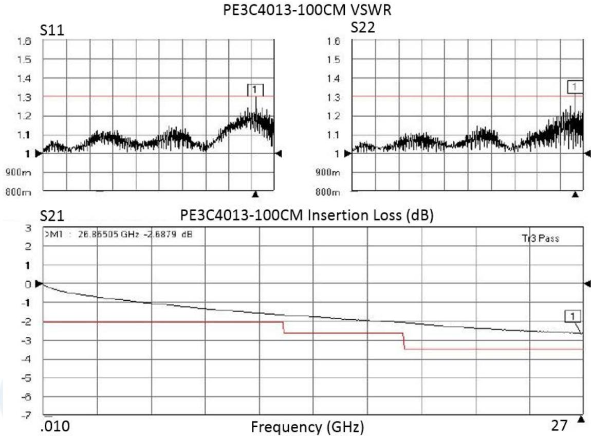
Click the following link (or enter part number in "SEARCH" on website) to obtain additional part information including price, inventory and certifications: [Handheld RF Analyzer Rugged Phase Stable Cable 3.5mm Female to 3.5mm Female Cable Using PE-FF430 Coax, RoHS PE3C4013](#)
