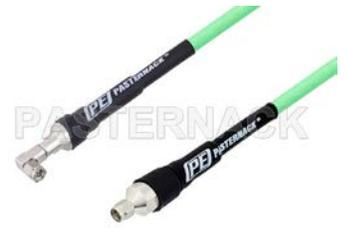
SMA Male to SMA Male Right Angle Low Loss Test Cable 50 cm Length Using PE-P300LL Coax, RoHS
