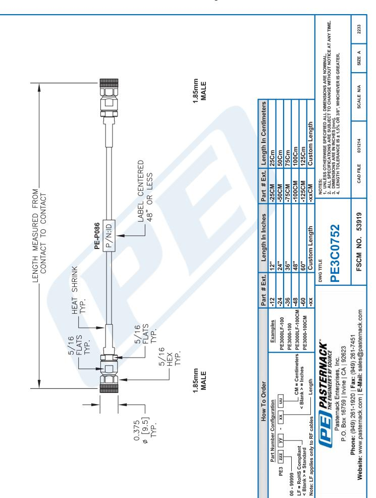
PE3C0752 CAD Drawing 1.85mm Male to 1.85mm Male Cable Using PE-P086 Coax
