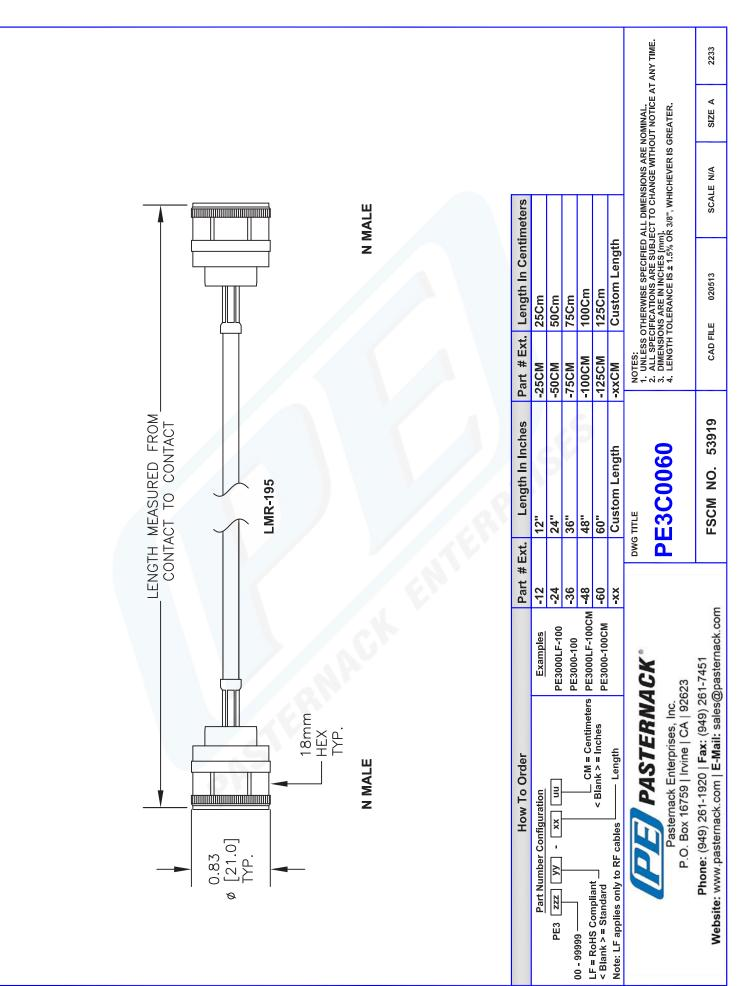
PE3C0060-48 CAD Drawing N Male to N Male Cable 48 Inch Length Using LMR-195 Coax
