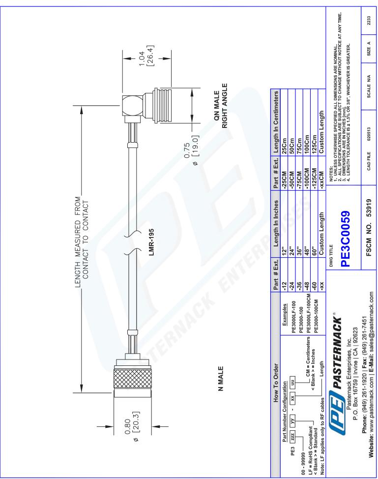
PE3C0059-24 CAD Drawing N Male to QN Male Right Angle Cable 24 Inch Length Using LMR-195 Coax
