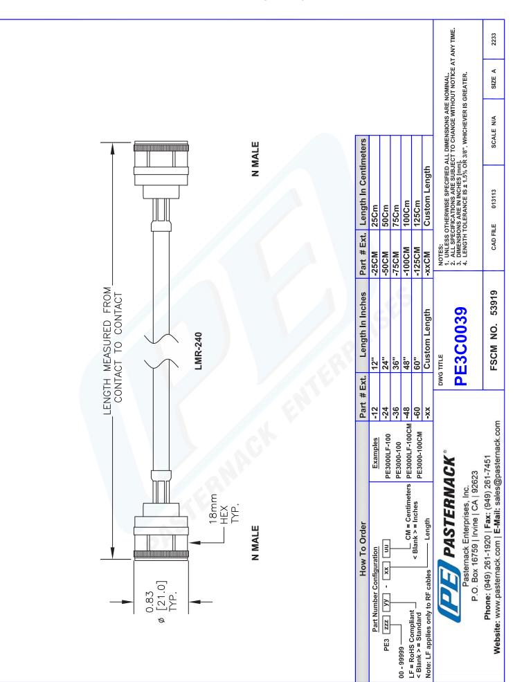
PE3C0039-60 CAD Drawing N Male to N Male Cable 60 Inch Length Using LMR-240 Coax
