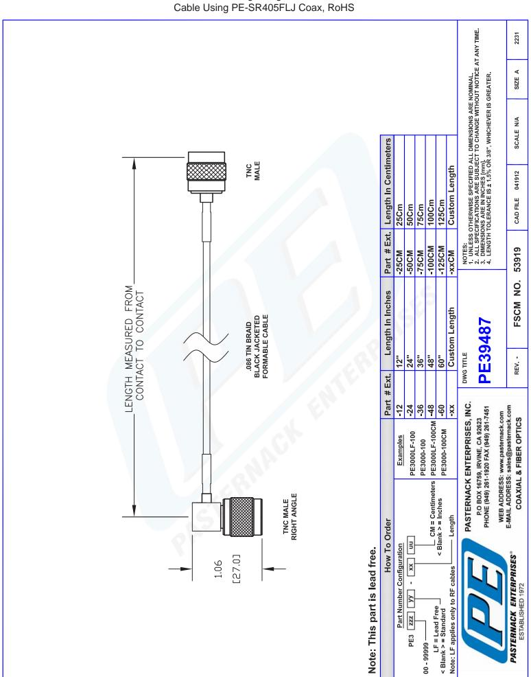
PE39487 CAD Drawing TNC Male to TNC Male Right Angle Semi-Flexible Precision
