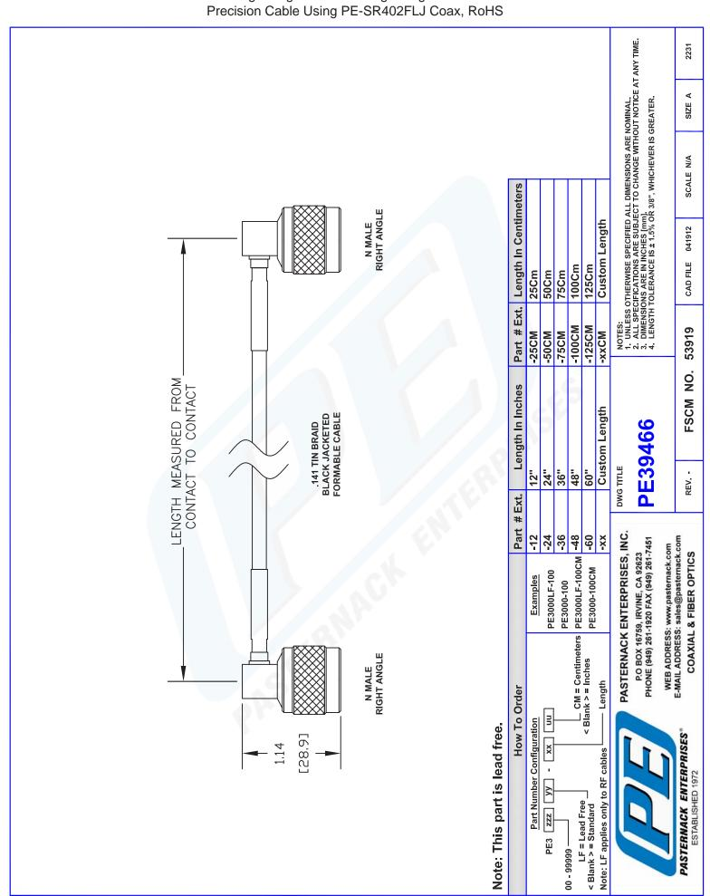
PE39466 CAD Drawing N Male Right Angle to N Male Right Angle Semi-Flexible
