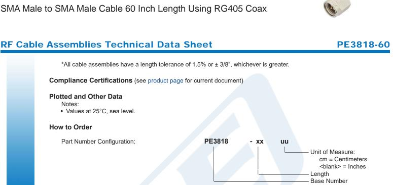
Example: PE3818-12 = 12 inches long cable PE3818-100cm = 100 cm long cable
