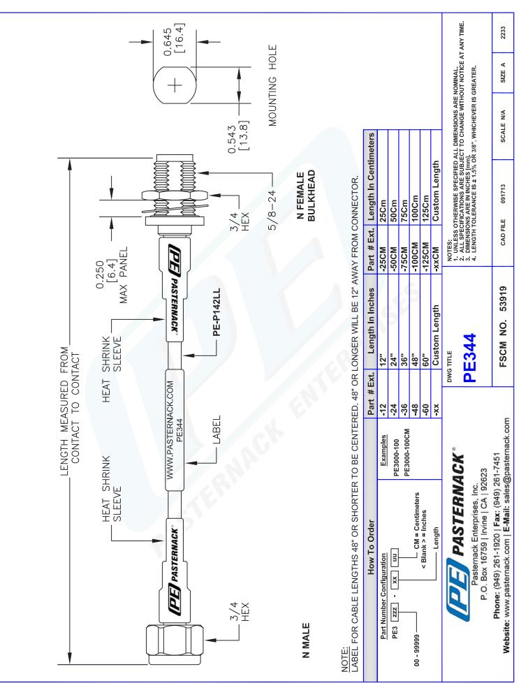
PE344 CAD Drawing N Male to N Female Bulkhead Low Loss Test Cable Using PE-P142LL Coax, RoHS
