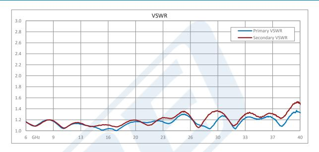
Directional 10 dB 2.92mm Coupler From 6 GHz to 40 GHz Rated to 30 Watts from Pasternack Enterprises has same day shipment for domestic and International orders. Our RF, microwave and millimeter wave products maintain a 99.4% availability and are part of the broadest selection in the industry.
