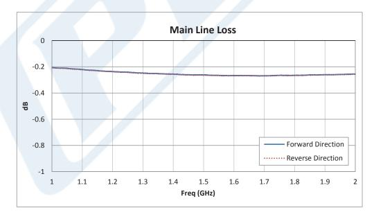
Click the following link (or enter part number in "SEARCH" on website) to obtain additional part information including price, inventory and certifications: Dual Directional 20 dB SMA Coupler From 1 GHz to 2 GHz Rated to 50 Watts PE2218-20
