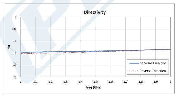
Click the following link (or enter part number in "SEARCH" on website) to obtain additional part information including price, inventory and certifications: Dual Directional 20 dB SMA Coupler From 1 GHz to 2 GHz Rated to 50 Watts PE2218-20
