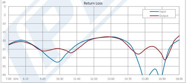
Click the following link (or enter part number in "SEARCH" on website) to obtain additional part information including price, inventory and certifications: Directional 10 dB SMA Coupler From 7 GHz to 18 GHz Rated to 50 Watts PE2212-10
