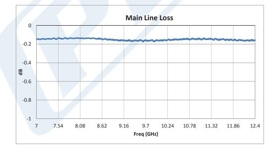
Click the following link (or enter part number in "SEARCH" on website) to obtain additional part information including price, inventory and certifications: Directional 30 dB SMA Coupler From 7 GHz to 12.4 GHz Rated to 50 Watts PE2205-30
