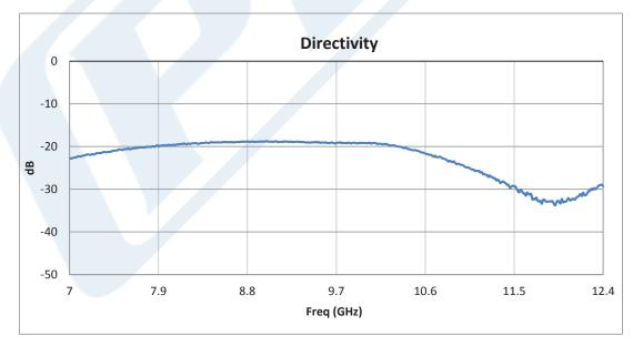
Click the following link (or enter part number in "SEARCH" on website) to obtain additional part information including price, inventory and certifications: Directional 20 dB SMA Coupler From 7 GHz to 12.4 GHz Rated to 50 Watts PE2205-20
