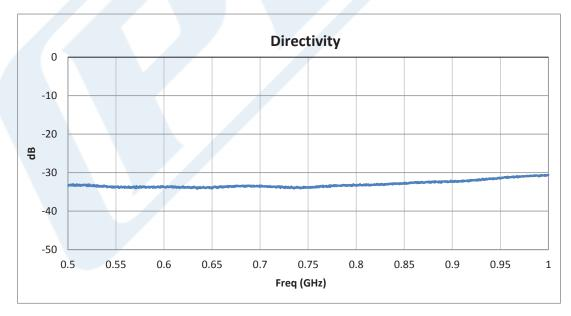
Click the following link (or enter part number in "SEARCH" on website) to obtain additional part information including price, inventory and certifications: Directional 20 dB SMA Coupler From 500 MHz to 1,000 MHz Rated to 50 Watts PE2200-20
