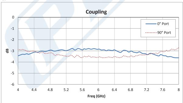
Click the following link (or enter part number in "SEARCH" on website) to obtain additional part information including price, inventory and certifications: 90 Degree SMA Hybrid Coupler From 4 GHz to 8 GHz Rated to 100 Watts PE2054
