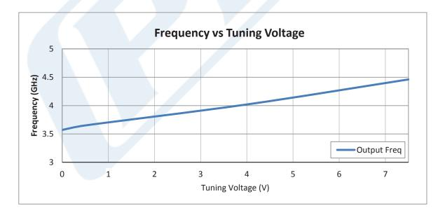
Click the following link (or enter part number in "SEARCH" on website) to obtain additional part information including price, inventory and certifications: Surface Mount (SMT) Voltage Controlled Oscillator (VCO) From 3.7 GHz to 4.35 GHz, Phase Noise of -83 dBc/Hz and 0.5 inch Hermetic Package PE1V13015
