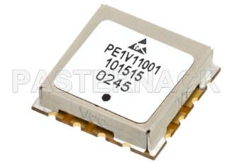
Surface Mount (SMT) Voltage Controlled Oscillator (VCO) From 18 MHz to 30 MHz, Phase Noise of -120 dBc/Hz and 0.5 inch Package
