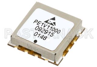
Surface Mount (SMT) Voltage Controlled Oscillator (VCO) From 10 MHz to 20 MHz, Phase Noise of -120 dBc/Hz and 0.5 inch Package
