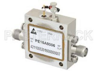
6 GHz to 12 GHz, Gain Block Amplifier, 12 dB
