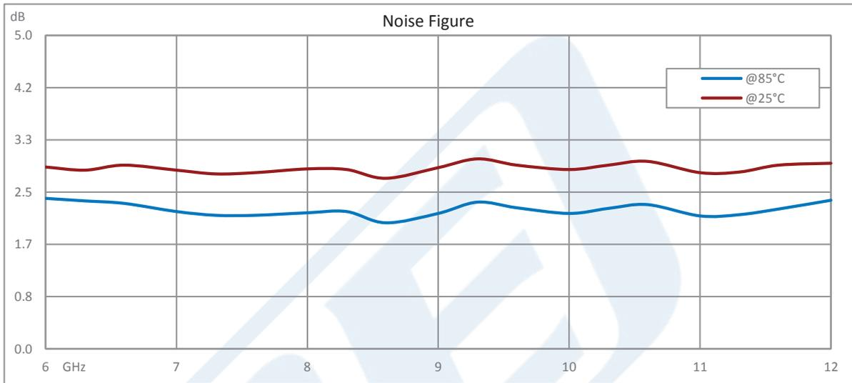
6 GHz to 12 GHz, Gain Block Amplifier, 12 dB Gain, 20 dBm IP3, 2.3 dB NF, SMA from Pasternack Enterprises has same day shipment for domestic and International orders. Our RF, microwave and millimeter wave products maintain a 99% availability and are part of the broadest selection in the industry.
