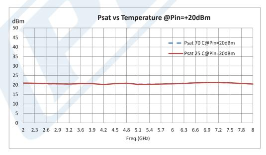
Click the following link (or enter part number in "SEARCH" on website) to obtain additional part information including price, inventory and certifications: 40 dB Gain, 19 dBm, 2 GHz to 8 GHz, Limiting Amplifier, -20 to 20 dBm Pin, SMA PE15A6008
