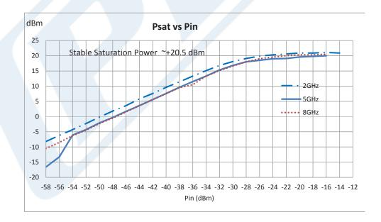
40 dB Gain, 19 dBm, 2 GHz to 8 GHz, Limiting Amplifier, -20 to 20 dBm Pin, SMA from Pasternack Enterprises has same day shipment for domestic and International orders. Our RF, microwave and millimeter wave products maintain a 99% availability and
