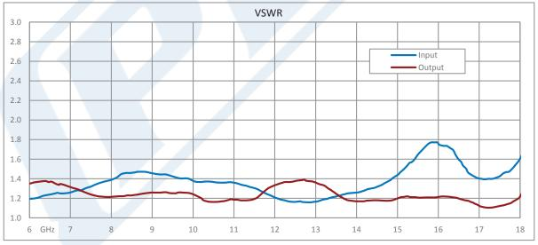
Click the following link (or enter part number in "SEARCH" on website) to obtain additional part information including price, inventory and certifications: 40 dB Gain, 10 Watt P1dB, 6 GHz to 18 GHz, High Power Amplifier, SMA, 46 dBm IP3 PE15A5050
