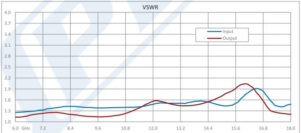
Click the following link (or enter part number in "SEARCH" on website) to obtain additional part information including price, inventory and certifications: 41 dB Gain, 5 Watt P1dB, 6 GHz to 18 GHz, High Power Amplifier, SMA, 44 dBm IP3 PE15A5049
