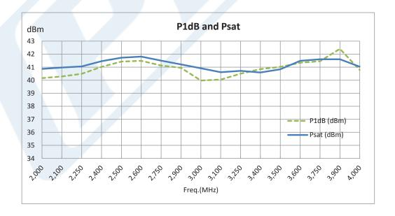
Click the following link (or enter part number in "SEARCH" on website) to obtain additional part information including price, inventory and certifications: 8 Watt Psat, 2 GHz to 4 GHz, High Power GaAs Amplifier, SMA Input, SMA Output, 39 dB Gain, 48 dBm IP3, Class A/AB PE15A5038F
