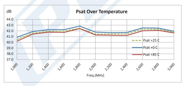
Click the following link (or enter part number in "SEARCH" on website) to obtain additional part information including price, inventory and certifications: 44 dB Gain, 8 Watt Psat, 1 GHz to 3 GHz, High Power GaAs Amplifier, SMA Input, SMA Output, 48 dBm IP3, Class AB PE15A5037
