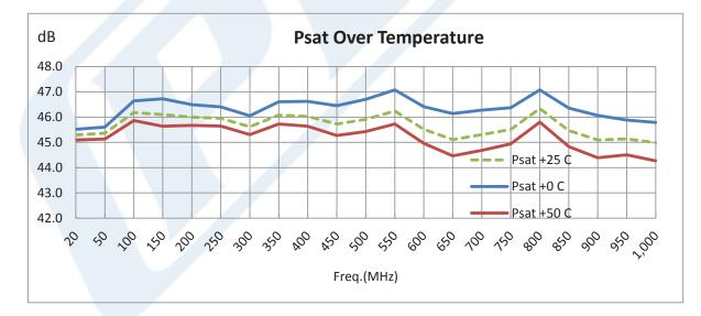
Click the following link (or enter part number in "SEARCH" on website) to obtain additional part information including price, inventory and certifications: 46 dB Gain, 25 Watt Psat, 20 MHz to 1 GHz, High Power LDMOS Amplifier, SMA Input, SMA Output, 48 dBm IP3, Class AB PE15A5031F
