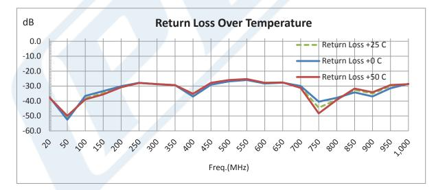
Click the following link (or enter part number in "SEARCH" on website) to obtain additional part information including price, inventory and certifications: 46 dB Gain, 25 Watt Psat, 20 MHz to 1 GHz, High Power LDMOS Amplifier, SMA Input, SMA Output, 48 dBm IP3, Class AB PE15A5031F
