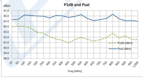
Click the following link (or enter part number in "SEARCH" on website) to obtain additional part information including price, inventory and certifications: 46 dB Gain, 25 Watt Psat, 20 MHz to 1 GHz, High Power LDMOS Amplifier, SMA Input, SMA Output, 48 dBm IP3, Class AB PE15A5031F
