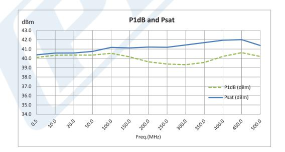
Click the following link (or enter part number in "SEARCH" on website) to obtain additional part information including price, inventory and certifications: 44 dB Gain, 8 Watt Psat, 0.5 MHz to 500 MHz, High Power LDMOS Amplifier, SMA Input, SMA Output, 42 dBm IP3, Class A/AB PE15A5029
