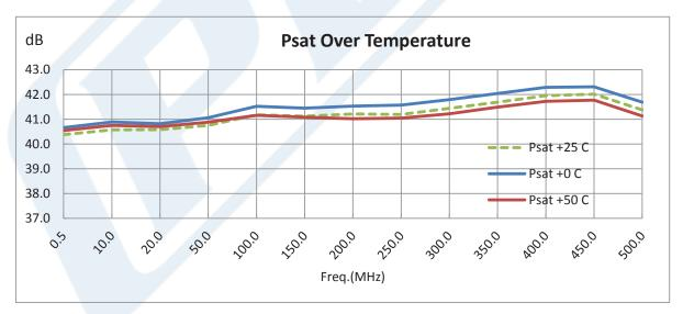
Click the following link (or enter part number in "SEARCH" on website) to obtain additional part information including price, inventory and certifications: 44 dB Gain, 8 Watt Psat, 0.5 MHz to 500 MHz, High Power LDMOS Amplifier, SMA Input, SMA Output, 42 dBm IP3, Class A/AB PE15A5029
