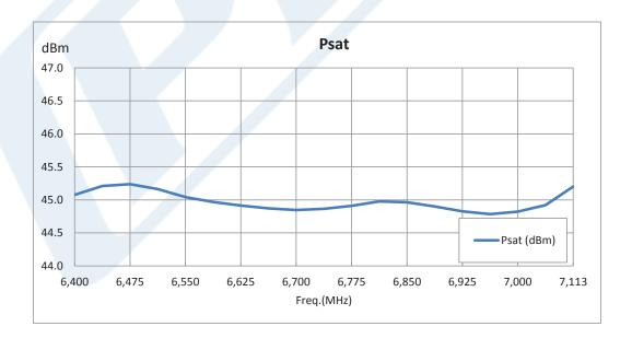
Click the following link (or enter part number in "SEARCH" on website) to obtain additional part information including price, inventory and certifications: 58 dB Gain, 20 Watt Psat, 6.4 GHz to 7.1 GHz, High Power GaN Amplifier, SMA Input, SMA Output PE15A5016
