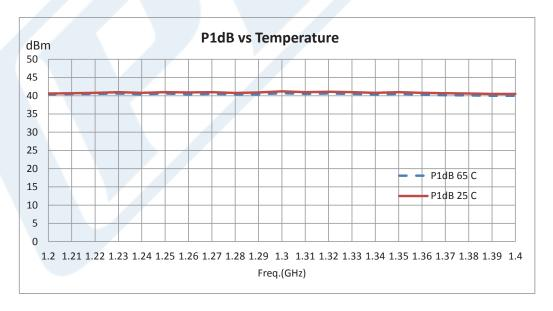
Click the following link (or enter part number in "SEARCH" on website) to obtain additional part information including price, inventory and certifications: 40 dB Gain, 10 Watt P1dB, 1.2 GHz to 1.4 GHz, High Power GaAs Amplifier, SMA Input, SMA Output PE15A5001
