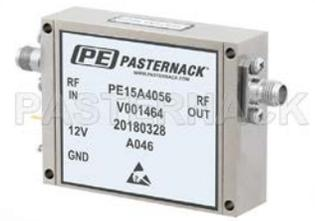
1 Watt P1dB, 2 GHz to 18 GHz, Medium Power Amplifier, SMA, 30 dB Gain, 37 dBm IP3
