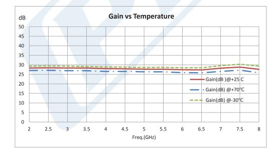
Click the following link (or enter part number in "SEARCH" on website) to obtain additional part information including price, inventory and certifications: 900 mW P1dB, 2 GHz to 8 GHz, Medium Power Broadband Amplifier, 33 dB Gain, SMA PE15A3016
