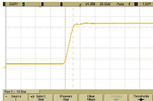
Rise Time at -54 Degrees C. 18GHz at 0dBm
