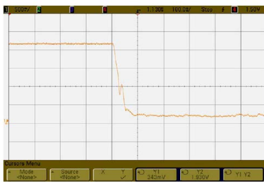
Recovery Time at 85 Degrees C. 18GHz at 0dBm
