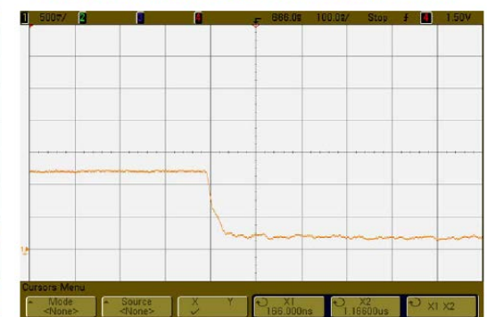
Recovery Time at 85 Degrees C. 18GHz at -20dBm
