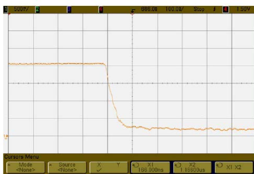
Recovery Time at 85 Degrees C. 18GHz at 0dBm
