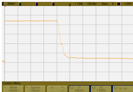
Recovery Time at -54 Degrees C. 18GHz at 0dBm
