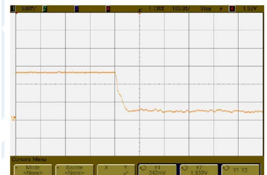
Recovery Time at 85 Degrees C. 18GHz at -20dBm
