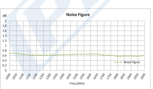
Click the following link (or enter part number in "SEARCH" on website) to obtain additional part information including price, inventory and certifications: 40 dB Gain, 25 dBm IP3, 0.8 dB NF, 11 dBm P1dB, 1 GHz to 2 GHz, Low Noise High Gain Amplifier SMA PE15A1019
